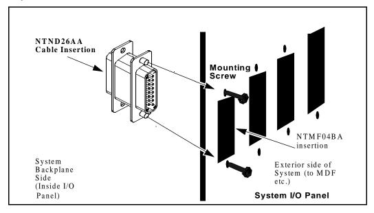
3 Obtain the correct length of the NTND26 DCHI Interface Cable Assembly to reach from the D-Channel port connector on the faceplate of the MSDL card to the outward side of the 15-pin filter connector installed in the I/O panel of the IPE Module that contains the DCHIP card. (See Figure 27)
